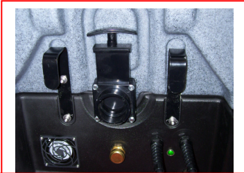
Remove four bolts holding valve assembly to flange fitting
