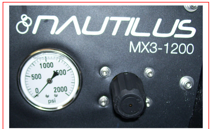
Pressure gauge & Regulator/Unloader
